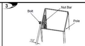
Insert one 3/8-16 x 1 1/4" bolt into the top hole, leave 1/2" of the thread exposed.
