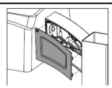
Feed supply wires into arm wiring chamber.
