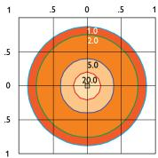
LPF4 105W - 25' Mounting Height, 0° Tilt Mounting Height 35 30 25 20 15 Multiplier 0.50 0.68 1.0
