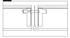
Raise next fixture to cantilever bracket and insert the joiner aligners into the corresponding slots on the already installed fixture.
