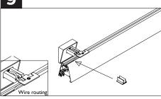
Run power cable down fixture channel and through power plate at the end of the fixture. Secure power cable into fixture channel using supplied cable clips at 4" increments.
