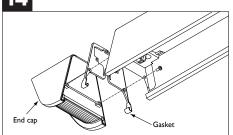
Snap on the gasket to the end of the fixture and attach end caps using supplied #8
