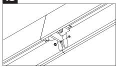
Join fixtures using supplied #8 screws and lock-nuts. Repeat steps 8-12 for each fixture in run.
