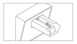
Slide on Wall covers and use supplied #8 lock-nut to secure to cantilever bracket (non-power mount shown).
