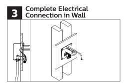
(Power locations only) Feed power cable through ½" hole in mounting bracket. Complete electrical connection to junction box through square cut out in mounting bracket.
