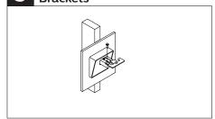
Attach fixture hanging brackets to cantilever brackets using supplied ¼"-20 bolts. Do not fully tighten.
