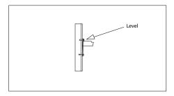
Attach brackets to wall using appropriate hardware (1/4" fastener recommended). Insure structure can support the weight of the fixture at 3.5lbs/ft. Install using two center holes for non-power locations and use 4 outer holes for power locations. Power locations require a vertically oriented 2"x4" recessed utility box (supplied by others). Use a spirit level and adjust mounting screws to level brackets.
