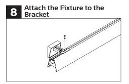
Raise fixture to brackets and use the supplied countersunk screw with countersunk washer to attach the fixture to the bracket. Adjust fixture hanging brackets so fixture is flush with cantilever arm and tighten.
