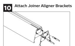
On the floor, slide variable mount bracket into next fixture in run. Attach joiner-aligner brackets into opposite side.
