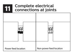
Complete power connections between fixtures.
