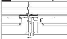
Raise next fixture to ceiling and insert the joiner aligners into the corresponding slots on the already installed fixture.
