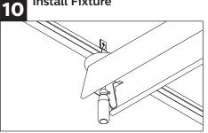
Using the supplied 1/4"-20 nuts attach the fixture to the ceiling through the slots in the top of the fixture. DO NOT FULLY TIGHTEN. The mount should be able to slide, but be snug.
