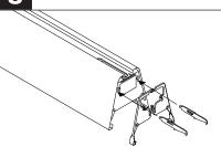
On the floor, slide variable mount bracket into next fixture in run. Attach joiner-aligner brackets, power plate and plug into opposite side.
