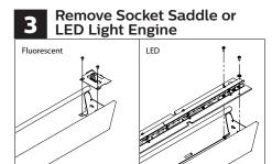
Remove socket saddle or LED light engine to gain access to mounting channel. When removing LED light engine be sure to disconnect the low voltage wire harness.
