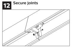
Join fixtures using supplied #8 screws and lock-nuts.
