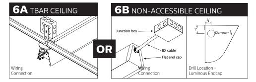
For non-accessible ceilings, drill 7/8" hole (location marked on Flat endcap: see diagram on right for drill location on Luminous endcap). Attach armored cable from the junction box (supplied by others) according to code.
