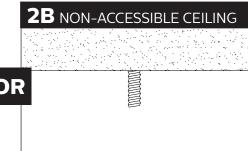
For non-accessible ceilings install 1/4"-20 stud extending 1/2" from ceiling. (see Mount Spacing Diagram on Page 1).
