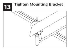
Tighten mounting bracket. Reinstall socket saddles or LED modules (remember to reconnect the low voltage wire harness). Install power plate and plug.
