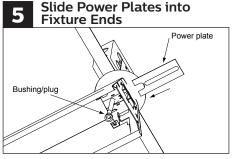
Slide power plates into fixture ends. Slide the supplied bushings over the SVT cord and snap into the power plate. If it is a non power location plug the hole with supplied plug bushing.
