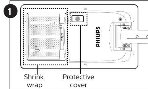
Remove shrink wrap and protective cover before installation.
