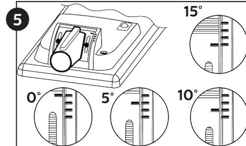
For accurate angle positioning, match pole marks mounting piece marking with luminaire marking
