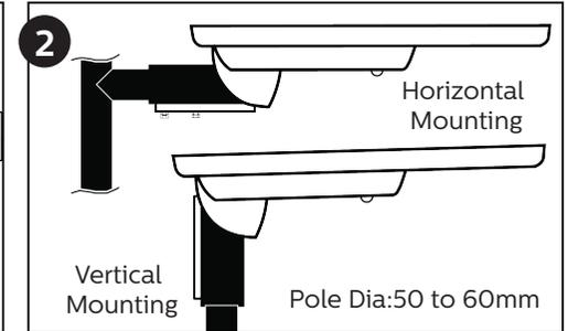
Mount the luminaire with pole, tighten the bolts with torque of 8 Nm.
