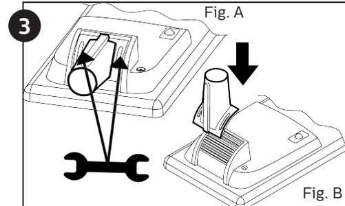
For vertical mounting unscrew and remove pole mounting bracket and assemble it as shown in Fig. B.
