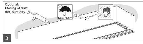
Mount CR250B IP65 luminaire in bracket acc.
