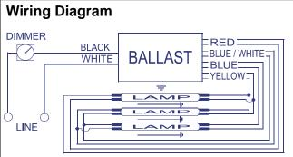
The wiring diagram that appears above is for the lamp type denoted by the asterisk  $(\ensuremath{^*})$
