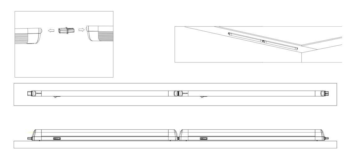
Inter connect two battens with the provided direct connector as depicted. Caution: Linkage battens (model&mode2) (max. upto eight battens)
