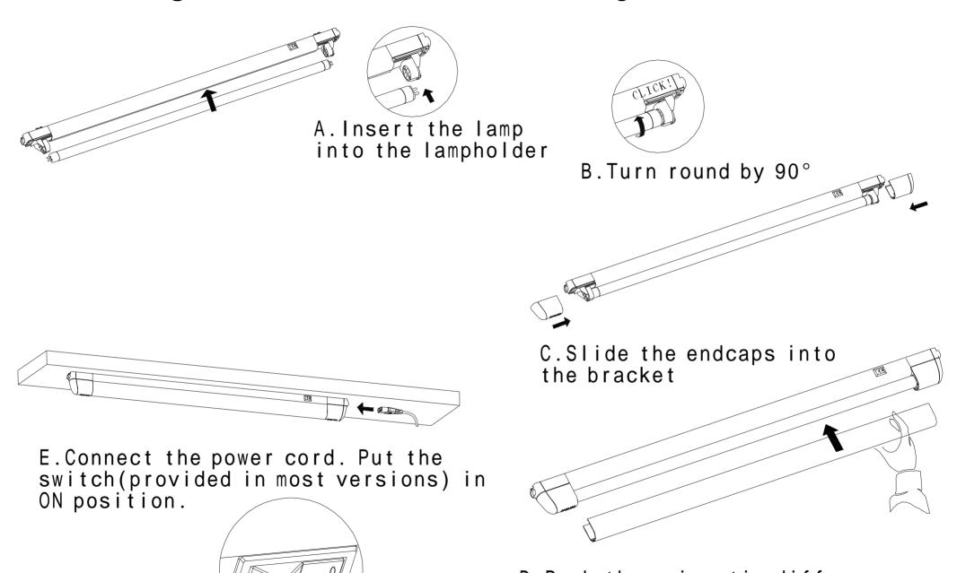
D. Push the prismatic diffuser back into the channel
