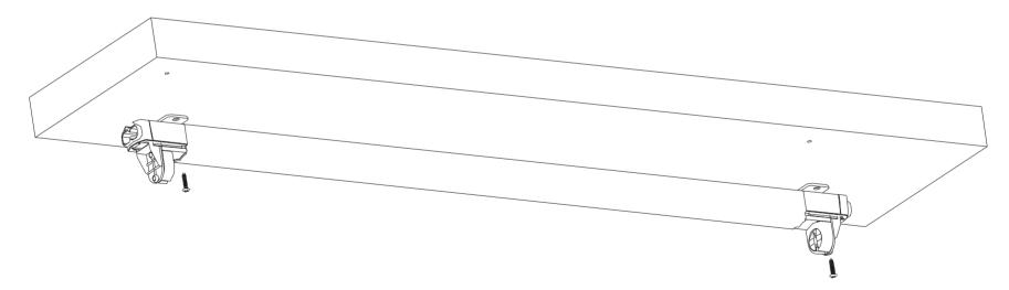
Twist off the screws (on the installer) and take off the batten.
