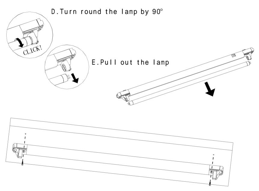
F. Twist off the screws (through the screw guides) and take off the batten.
