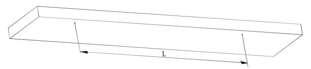
Pre-drill the holes on the ceiling/wall, at an appropriate distance as below:
