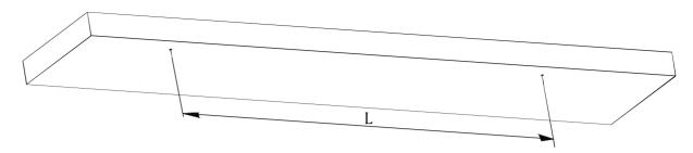
Pre-drill two holes on the ceiling/wall, at an appropriate distance as below:
