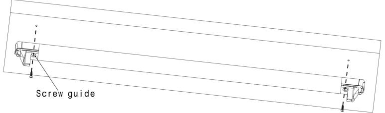
Firmly fix the batten (through the screw guide) with provided screws on the ceiling/wall.
