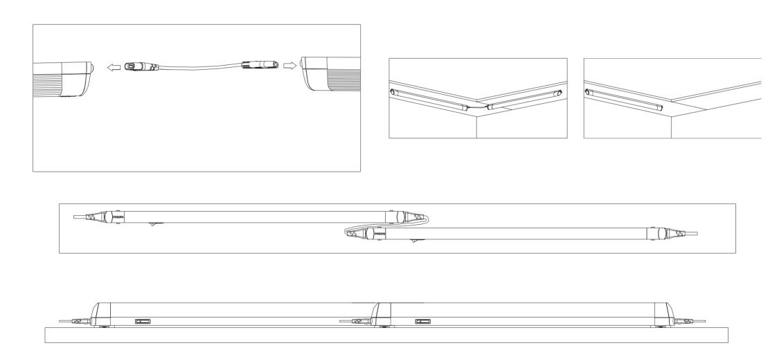
Inter connect two battens with the provided connector as depicted.
