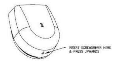
(2): Remove electronics module from backplate by inserting a flat bladed screwdriver between backplate and module and prying module away from backplate.
