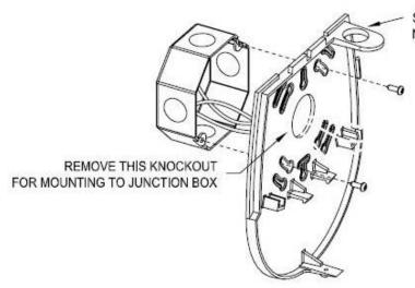
SECURE SURFACE CONDUIT TO THIS FLANGE IF NOT USING A JUNCTION BOX FOR MOUNTING
