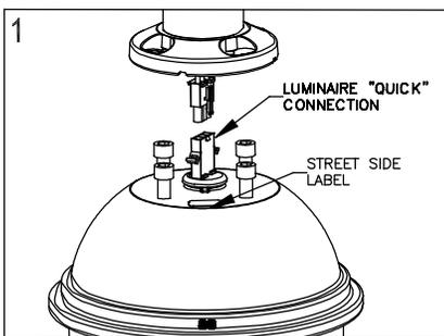
1. Lift the luminaire under the cast-suspension ring. Align with street side on luminaire. Connect the quick-disconnect terminals and push the connection in the mounting opening. Soulevez le luminaire sous l'anneau de fixation. Aligned with the street side indicated on the luminaire. Connect the quick-disconnect terminals and push them into the mounting opening.
