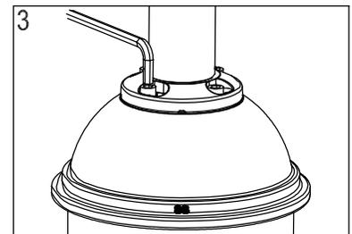
3. Tighten all four screws to firmly secure the luminaire in place. Torque: 240 lbs.in, 20 lbs.ft. Serrez les 4 boulons pour fixer le luminaire. Couple de serrage; 240 lbs/po, 20 lbs/pi
