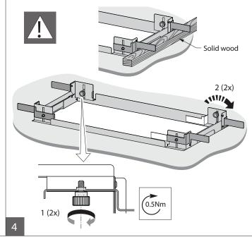
V-clips are pre-mounted when ordered with luminaire.
