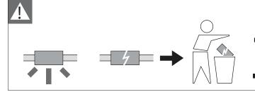
The light source of this luminaire is not replaceable; when the light source reaches its end of life the whole luminaire shall be replaced.
