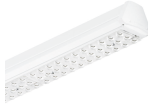
Maxos Led Industry - Generation 4 - 1 unit for TL5 49 W - LED Module, system flux 6600 lm - 840 neutral white - Power supply unit with DALI interface and constant light output - Wide beam - Constant light output - Connection unit 5-pole - White
