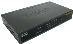
Unmanaged switch 4 POE port, 48 V
