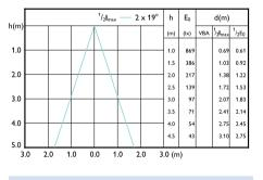
Beam diagram - ESS LED MR16 4.5-50W 36D 830 100-240V
