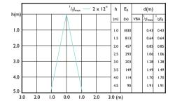
Beam diagram - ESS LED MR16 3-35W 36D 830 SO 100-240V
