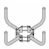
Steel Bracket, Wrap Around, Quad Spider, Wood Pole
