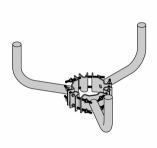
Steel Bracket, Wrap Around, Triple Spider, Wood Pole
