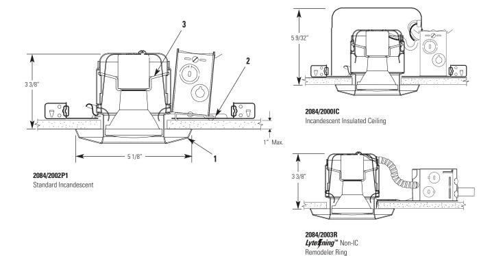
Complete Fixture consists of Frame-In Kit & Reflector Trim. Select each separately.
