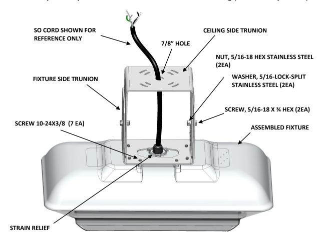
The SO cord can then be routed to the junction box and connected
