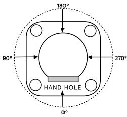
For Factory Installed Options and Accessories, Specify Orientation from Hand Hole and Height Above Pole Base Where Required.
