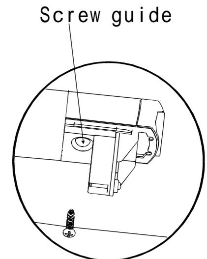
Firmly fix the batten (through the screw guide) with provided screws on the ceiling/wall.
