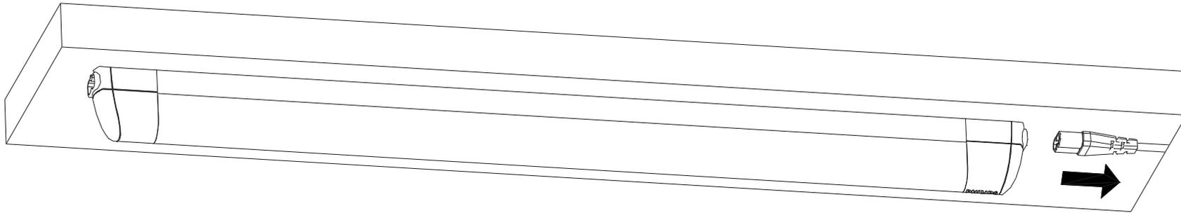
Switch off and pull out the power cord
