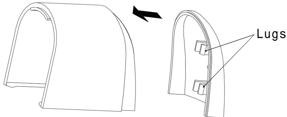
Click fit the new bezel onto the endcap gently- ensuring that the lugs fit properly into the sockets.
