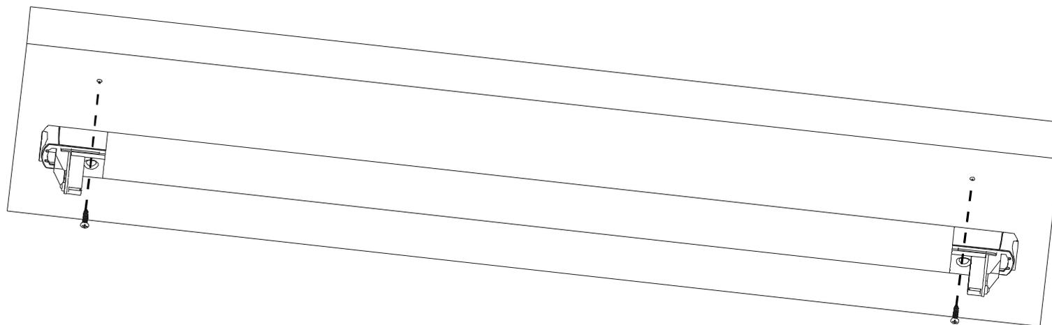
F. Twist off the screws (through the screw guides) and take off the batten.
