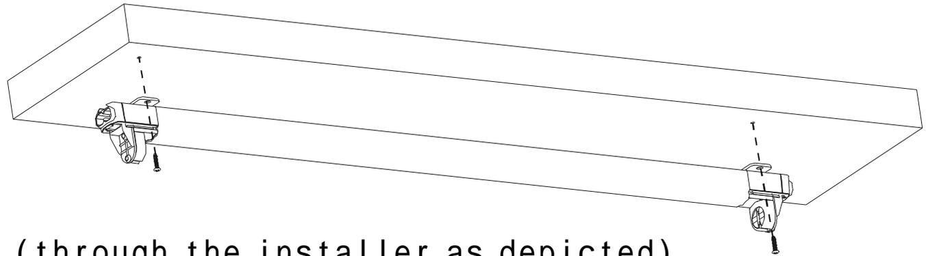
Firmly fix the batten (through the installer as depicted) with provided screws on the ceiling/wall.
