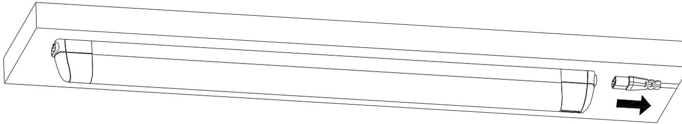
A. Switch off and pull out the power cord
