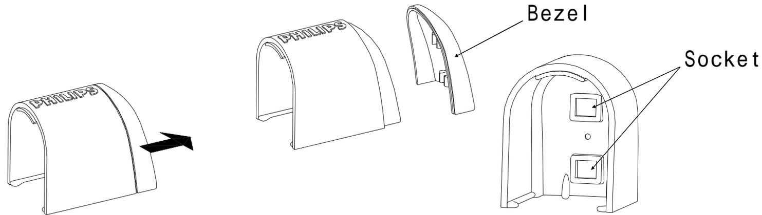
Pull out the metallised bezel from the endcap gently
