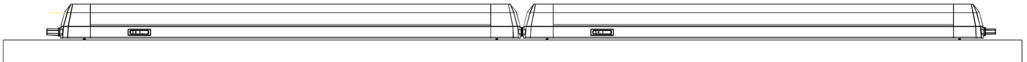
Inter connect two battens with the provided direct connector as depicted.
