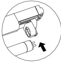
A. Insert the lamp into the lampholder
