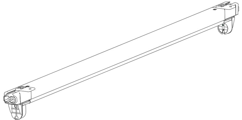
Slide in the installers into the channel groove, till the end
