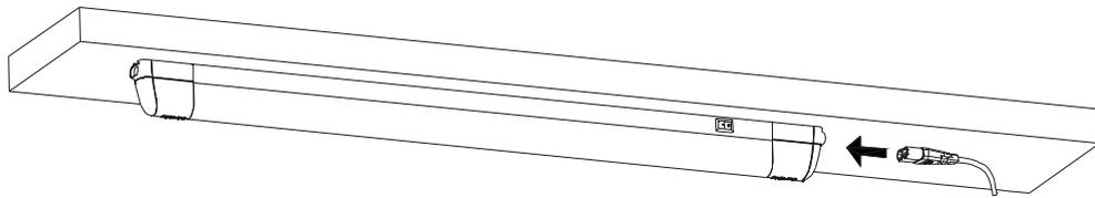
E. Connect the power cord. Put the switch (provided in most versions) in ON position.
