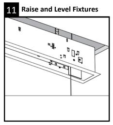
Once the power connections are complete, pull the aircraft cable to raise all modules to just below the ceiling.
