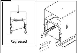
**Regressed Lens**: Angle lens to insert into fixture. Lay lens on aluminum extrusion flange.
