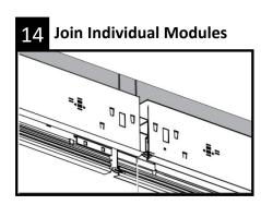
Gently slide housing modules together, ensuring joiner aligners are engaged inside the trim in the adjacent module.
