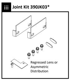
\*Note: One kit required for each joint. Joint kit determined by flush or regressed lens mounting and symmetric or asymmetric light distribution. Tools: Phillips screwdriver, 5/16" Nut Driver
