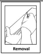
**Flush Lens:** Snap in lens into fixture. Lens Removal: To remove snap-in lens for maintenance purposes, insert a flat, smooth edged object between lens and housing. Twist to release pressure and remove lens.
