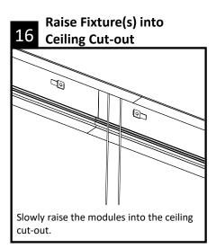
Important: For continuous row modules, start at one end and gradually raise each module up one inch at a time. Repeat process until housing is fully recessed and housing trim touches drywall ceiling. Do not stress the joint connection by tilting the module, as damage can occur.
