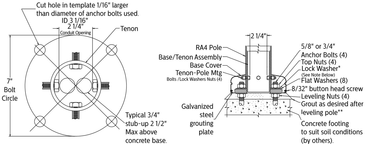
NOTE: Internal clearance of tenon/pole mounting bolts dictates allowable area for stub-ups.
