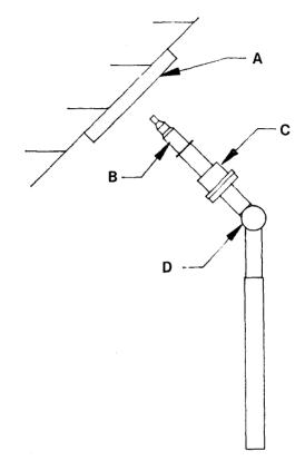
The sloped ceiling adapter is now ready for insertion of Focal Jacks or Extender Stems.
