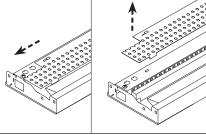
Shift top reflector to the left and then remove the reflector.
