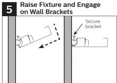
With 2 people, raise fixture into position and engage it on hooks located on top of wall brackets, then rotate it down into position. Secure bracket using supplied hardware.
