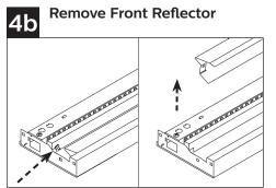
Remove the screws holding the front reflector and then remove the front reflector.
