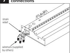
Complete electrical connections using wire nuts (supplied by others). Re-install pan and hardware removed in STEP 6.
