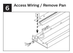
To access wiring, remove screw from top pan and lift pan off. Apply strain relief to power cord.
