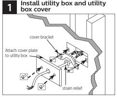
Determine power feed location and install 2"x4" utility box (supplied by others) parallel with fixture. Complete connections at utility box with supplied power cord. Attach cover bracket using supplied hardware. Punch power access hole in supplied cover, feed power cord through and attach strain relief on wall side. Attach cover using supplied painted hardware.
