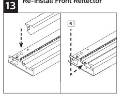
Re-install front reflector using short (stubby) screwdriver.
