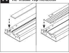
Identify smooth side of the Light Guide and ensure it is installed smooth side DOWN.
