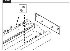
Attach endcap to first and last module in each row using supplied hardware.
