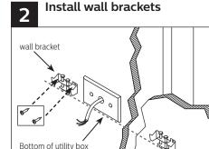
should be in line with bottom of wall brackets.
