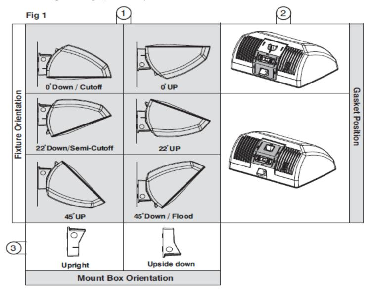
NOTICE: Fixture is listed under UL Standard #1598, for wet locations. It is not intended for use in car washes, hose down areas, or in direct contact with lawn sprinklers or roof runoff. In addition, this fixture should not be mounted in elevated ambient areas or areas that may entrap heat (i.e.- indo or pools, saunas, etc.).
