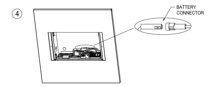
Connect red battery lead by pushing connector halves together (see above). Make AC service connections. See table below for wiring guide.
