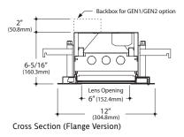
Note: The recommended ceiling opening for a single flange model is 10-7/8" x 48-5/16". Refer to the Installation Instructions for more detailed instructions including the ceiling opening size for multiple fixture installations.
