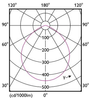
Light Distribution Diagram - DN060B LED8S/840 PSU WH
