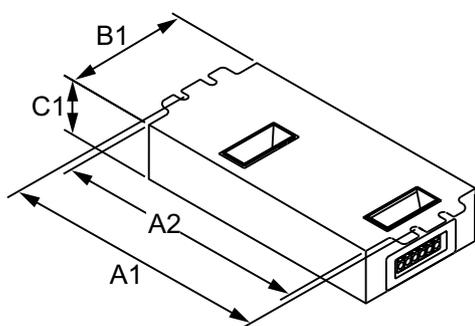
ELE DIM BALLAST (2) 42W CFL (4-PIN) 277V
