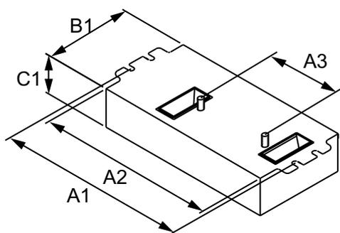
ELE DIM BALLAST (2) 18W CFL (4-PIN) 277V
