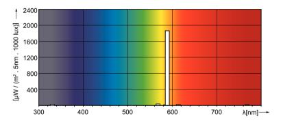
Spectral Power Distribution Colour - SOX 55W BY22d T50 1SL/12
