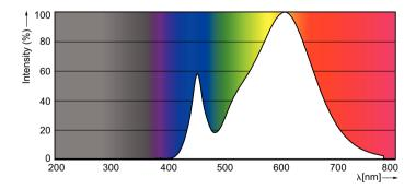
Spectral Power Distribution Colour - LED 60W E27 WW 230V R63 36D DIM 1BC/4
