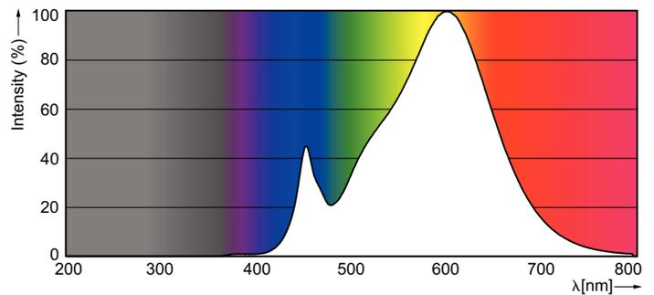
Spectral Power Distribution Colour - LEDBulb 9.5-70W E27 830 220-240V 3PF/10
