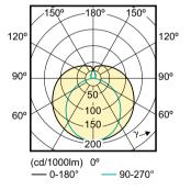
Light Distribution Diagram - CorePro LEDtube 600mm 9W 840 T8 C W G
