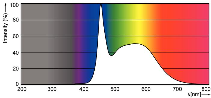
Spectral Power Distribution Colour - ESSENTIAL LEDtube 600mm 9W 865
