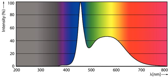
Spectral Power Distribution Colour - LEDCLA 50W GU10 865 220-240V 36D ND1BC/6
