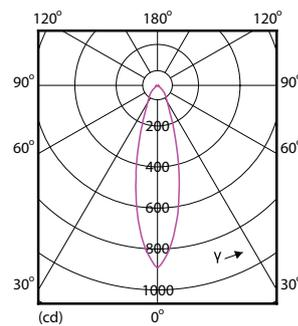
Light Distribution Diagram - 7PAR20/LED/F25/840/E26/GL/DIM 120V
