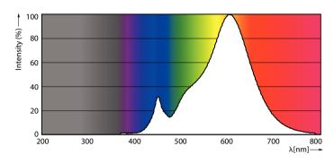
Spectral Power Distribution Colour - MAS LED spot VLE D 5.5-35W MR16 827 36D
