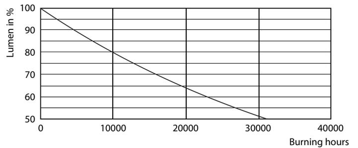
Lumen Maintenance Diagram - CLA LEDBulb ND 8-75W E27 CW A60 CL
