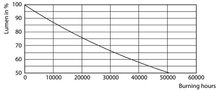
Lumen Maintenance Diagram - LEDBulb 5W E27 3000K W A19 1PF/6 MX
