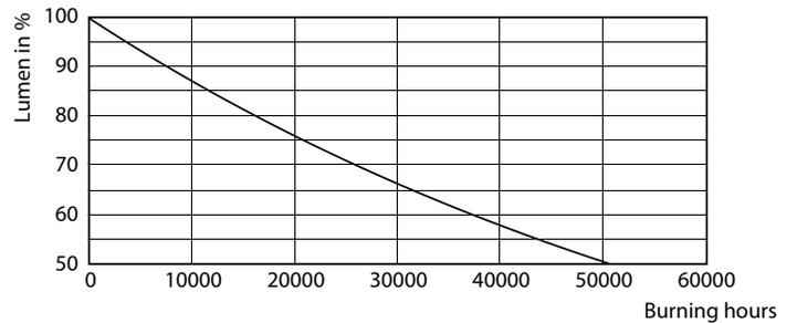
Lumen Maintenance Diagram - LEDBulb 9W E27 6500K W A19 1PF/6 MX
