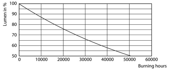
Lumen Maintenance Diagram - LEDBulb 10W E27 6500K W A19 1PF/6 MX
