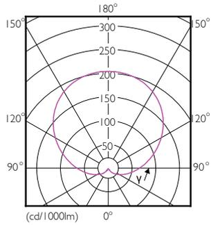
Light Distribution Diagram - LEDBulb 10W E27 6500K W A19 1PF/6 MX
