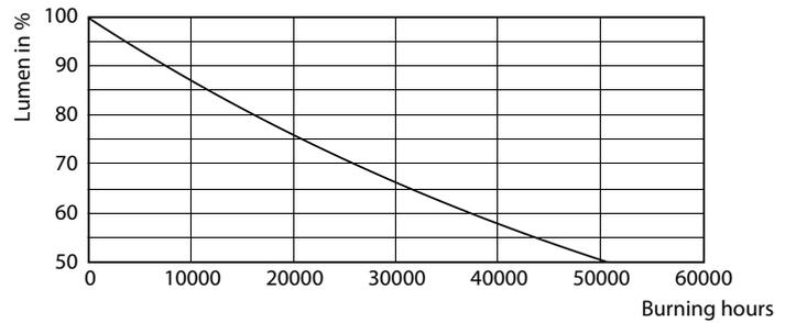
Lumen Maintenance Diagram - LEDBulb 14W E27 3000K W A21 1PF/6 MX
