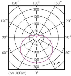
Light Distribution Diagram - LEDBulb 25W E27 6500K W A35 1PF/6 MX
