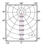
Light Distribution Diagram - 33PAR38/PER/830/S15/DIM/120V 6/1FB
