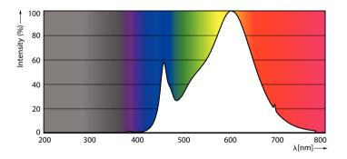
Spectral Power Distribution Colour - 33PAR38/PER/830/S15/DIM/120V 6/1FB
