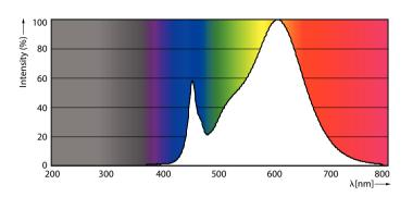
Spectral Power Distribution Colour - 13T8-6U/MAS/24-830/IF20/P/DIM 10/1
