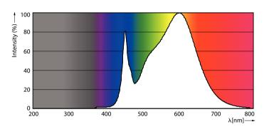
Spectral Power Distribution Colour - 13T8-6U/MAS/24-835/IF20/P/DIM 10/1
